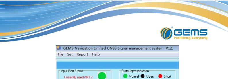
If the antenna open or short circuit, the front panel of the machine GPS Locked green light is off, Alarm red light flashes to indicate alarm, PC-side reading antenna operating state shorted or opened.
